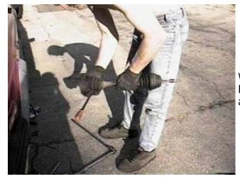
With the 6 bolts remove, the half axle is free from the car. From this point, it is just the reverse to reinstall. For me, I am now ready to install a new CV boot.
