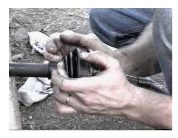
The smaller end of the CV boot will need to be clamped over these ridges. These help keep the CV boot in place.
