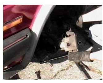
As you can see here, you can pull the strut/brake asm out quite a bit so you can remove the CV axle from it.
