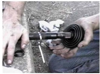
Once you've cleaned out the CV joint, set it aside. With a old rag, wipe clean the axle shaft. Then slide on the smaller metal band that came with the CV boot, and next the CV boot itself.
