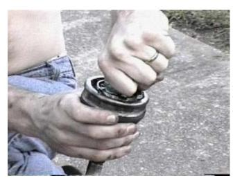
Now take the CV grease that came with the CV boot, cut a small hole it it. I cut off a corner of the bag and then stuff that corner into the opening of the CV joint and squeeze the grease in until I see if ooze out around the edges.
