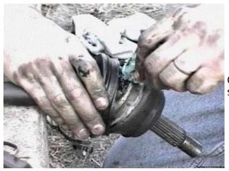
Once you clamp the smaller part of the CV boot in place, squeeze the rest of the CV grease into the CV boot.
