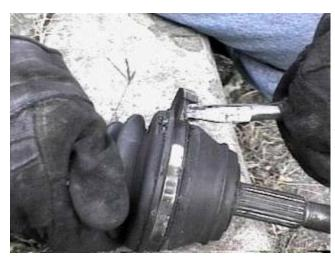
Using my side cutters (dikes), I'm removing the metal bands that keep the CV boot in place. Once those are gone, I'll cut the old CV boot off.
