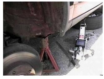
Remove the wheel and support the car as shown in the link above..
