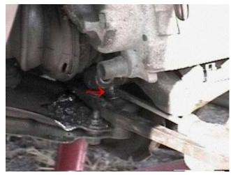
Using a pry bar or large screw driver, loosen the ball joint from the knuckle. You are just wanting to make sure they aren't stuck together once the bolt has been removed. As you can see where the arrow is pointing, I've moved it some and exposed some of the stud. Sometimes you have to use a hammer and hit the lower control arm to help jar things loose.
