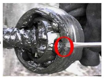
While using a bench top vice is nice, I didn't have one handy, so I'm standing on the half axle. Anyway, notice how I've got the CV joint tilted at an angle so the hammer will only strike the outer part of it. It only took a few taps to free it from the shaft.
