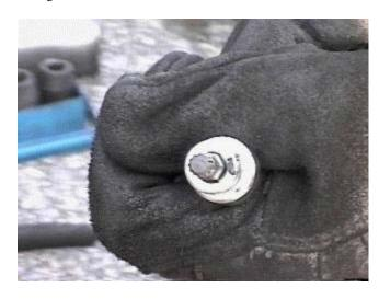
With that 12 point tool on the end of my 24" extension, I remove the 6 bolts.
